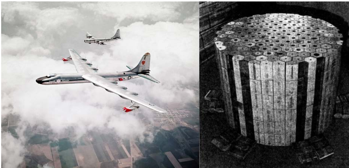
Figure 1-1 LEFT – Convair NB-36H nuclear test aircraft flew with an operating reactor in preparation for X-6 nuclear bomber program [image courtesy of US Air Force, US DOD]; RIGHT – BeO moderator for 1954 Aircraft Reactor Experiment (ARE) [image courtesy of ORNL, US DOE].
